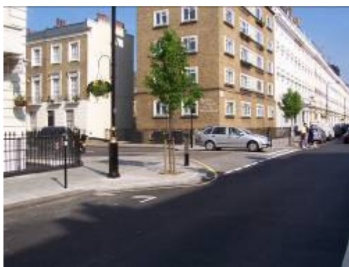
The use of a build out at junction allows for the pedestrian desire line to be respected.
