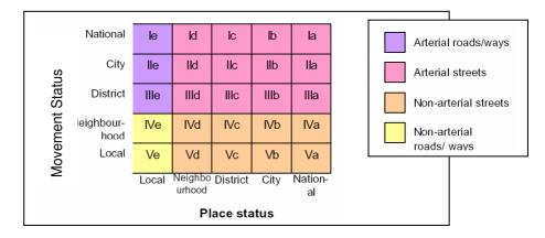
2.3.11 Using this matrix, it is possible to classify most types of road and street, for example:
