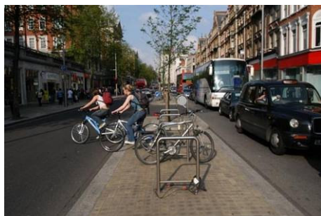
Cycle parking on central reservation
