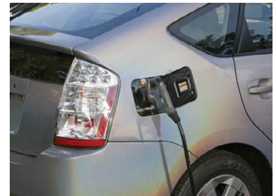
Figure 7. The Toyota Prius is an electric hybrid that provides substantial gains in fuel economy and major reductions in total tailpipe emissions. It uses 0.64 kWh of energy per passenger mile (given observed vehicle occupancy).
