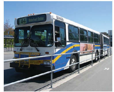
Figure 6. Shows an articulated diesel bus in service in Vancouver, BC that uses 0.56 kWh of energy per passenger mile (given observed vehicle occupancy).
