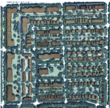
Figure 11-2 - The sprawling, status-quo street pattern (Figure 11-1) is less efficient than the compact traditional development (Figure 11-2). Narrow, interconnected streets save more land and make walking and cycling easier. Total daily vehicle kilometers travelled (VKT) in traditional development patterns can be up to 43% lower than status-quo development patterns.
