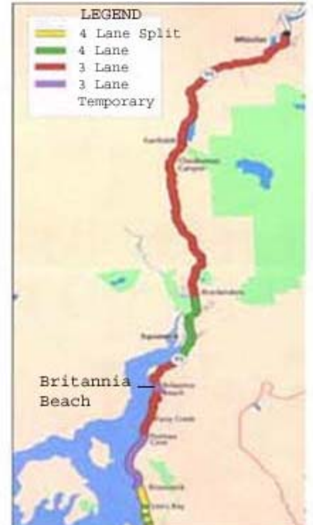
Sea to Sky Highway proposal showing short temporary 3-lane section at Britannia Beach Community Picture from: Sea-to-Sky Highway Improvements
